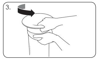
To remove the lid for emptying unscrew counterclockwise and lift off.
