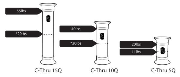
\* Glasdon recommends that the C-Thru 15Q and C-Thru 10Q are not filled beyond the mid-point of the body to improve handling and extend the lifetime of the product.
