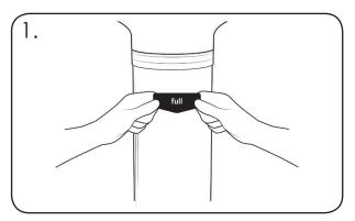
Fit the 'full' decal (if applicable). Remove the adhesive backing from the decal and apply the decal to the polycarbonate body in a suitable visible location (please refer to 'weight guide').
